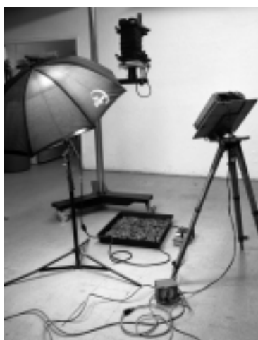
Figure 5. This image shows how the camera and projector and light were put together for the Flowers in Newsprint shot.
