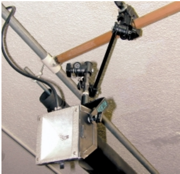
Figure 4. Mounting the main light source—a Smith-Victor 780 spotlight—on the studio ceiling.
