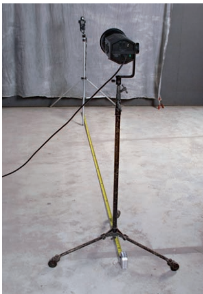
The meter and the strobe were 10 feet apart for the power test. The soft box was in the same position.
