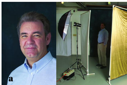
Figure 5. Umbrella has been moved slightly from figure 3, with the large silver reflector (a). The reflector is bouncing light directly from the umbrella, as seen in the setup (b).
