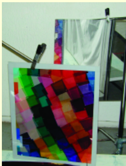
Figure 3. This shot shows the filter made from a swatch book. It also shows the large Plexiglas reflector that sends light through the filter.
